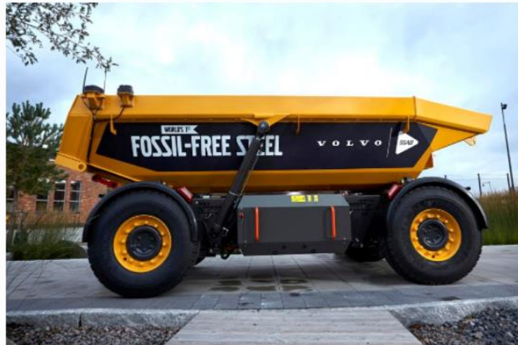
Volvo's load carrier is autonomous, fully electric and made using fossil fuel-free steel. © AB VOLVO
